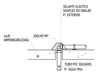
**12** DETALHE - COLUNA DE ÁGUA FRIA NA LAJE
